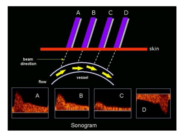
**Figure 3:** Effect of the Doppler angle in the sonogram. (A) higher-frequency Doppler signal is obtained if the beam is aligned more to the direction of flow. In the diagram, beam (A) is more aligned than (B) and produces higher-frequency Doppler signals. The beam/flow angle at (C) is almost 90° and there is a very poor Doppler signal. The flow at (D) is away from the beam and there is a negative signal.
