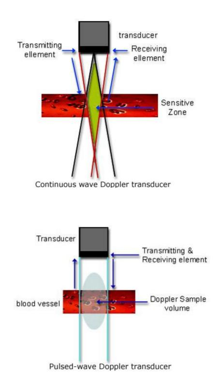
Figure 4: Illustration of continuous wave and pulsed wave Doppler.
