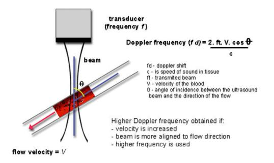
**Figure 2:** Doppler ultrasound. Doppler ultrasound measures the movement of the scatterers through the beam as a phase change in the received signal. The resulting Doppler frequency can be used to measure velocity if the beam/flow angle is known.
