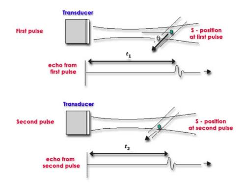
**Figure 1:** Ultrasound velocity measurement. The diagram shows a scatterer S moving at velocity V with a beam/flow angle. The velocity can be calculated by the difference in transmit-to-receive time from the first pulse to the second (t2), as the scatterer moves through the beam.
